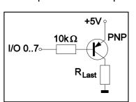
flows only when L-level is applied. A single pin may be loaded with max. 10mA, all pins together may be loaded with 26mA in all, i.e. 2 pins @ 10mA plus 1pin @ 6mA. Its possible i.e. to connect and switch a LED
