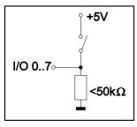
Input pins accept voltage levels between -0,5V and +0,2V\*VDD-0,1V. Leakage current is max.  $\pm 10\mu A$ . Trigger levels are listed in table of technical description on page 3. Command "X n1" allows read in of datas on each individual pin IO 0..7. Voltage level must be stable all over read in procedure. There is no built in debounce function.
